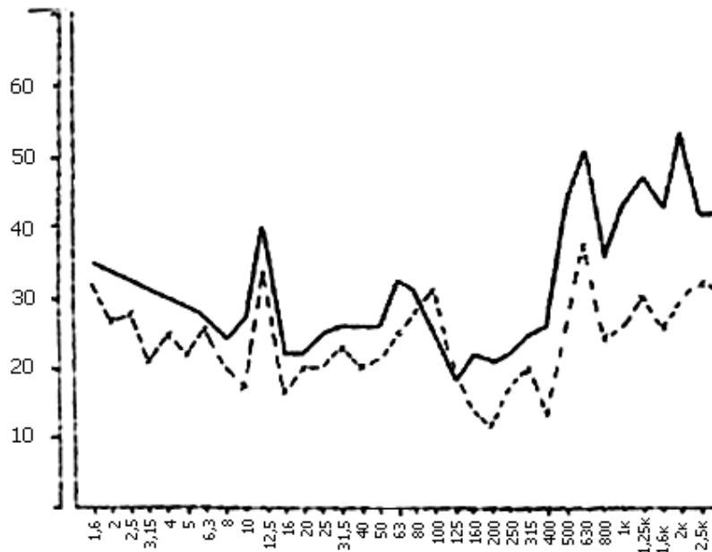
Figure 2. 1/3 octave spectrum of vibration displacement of compressor N 9/01 KuibyshevAzot public joint stock company in point 3, direction y (during operation load and without load)
