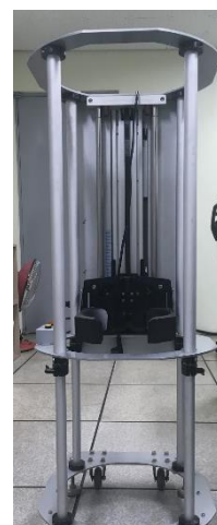
Figure 1 Automated rubber ball drop device
