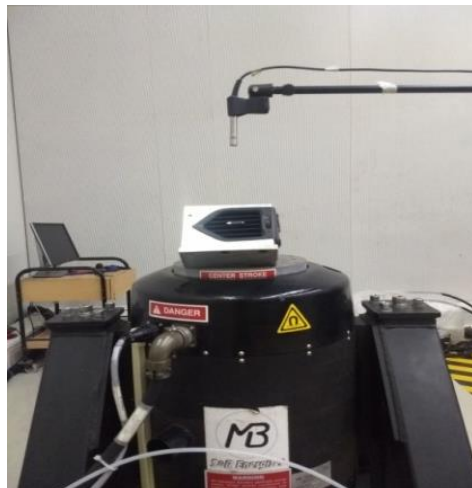
Figure 1. Electromagnetic shaker used in vibration test
