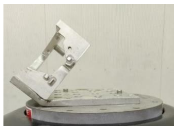
Figure 2. Air vent fixture used in BSR test
