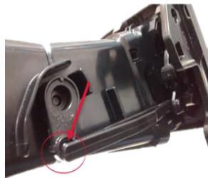
Figure 6. Knob link free play location observed in test sample
