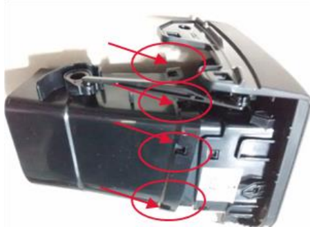
Figure 7. Air vent housing free play locations observed in test sample
