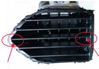
Figure 5. Horizontal vane free play locations observed in test sample
