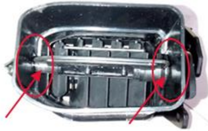
Figure 4. Damper shut off flap free play observed in test sample
