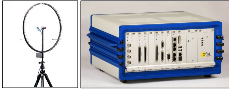
Figure 2 – Ring microphone array and data recorder used in the measurements.
