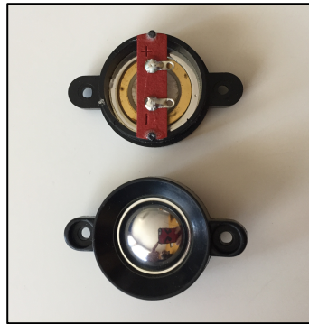
Figure 3 – Ultrasonic piezo speakers used in the measurements
