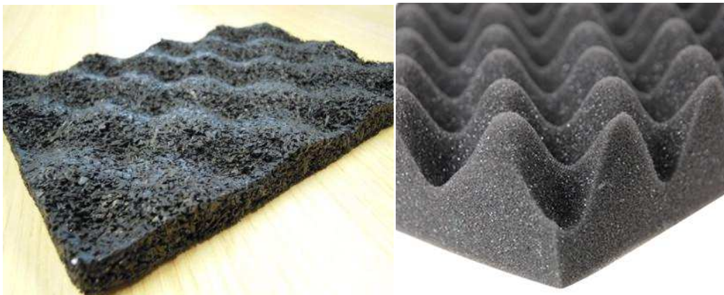
Figure 1 : Examples of a shaped porous materials used for vibration insulation.
