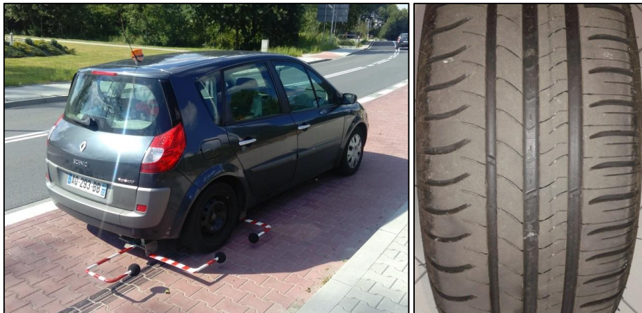
Fig. 1. CPX measuring system no. 1 – French car Renault Scenic (left) and the test tyre used – Michelin Energy Saver+ (right)
