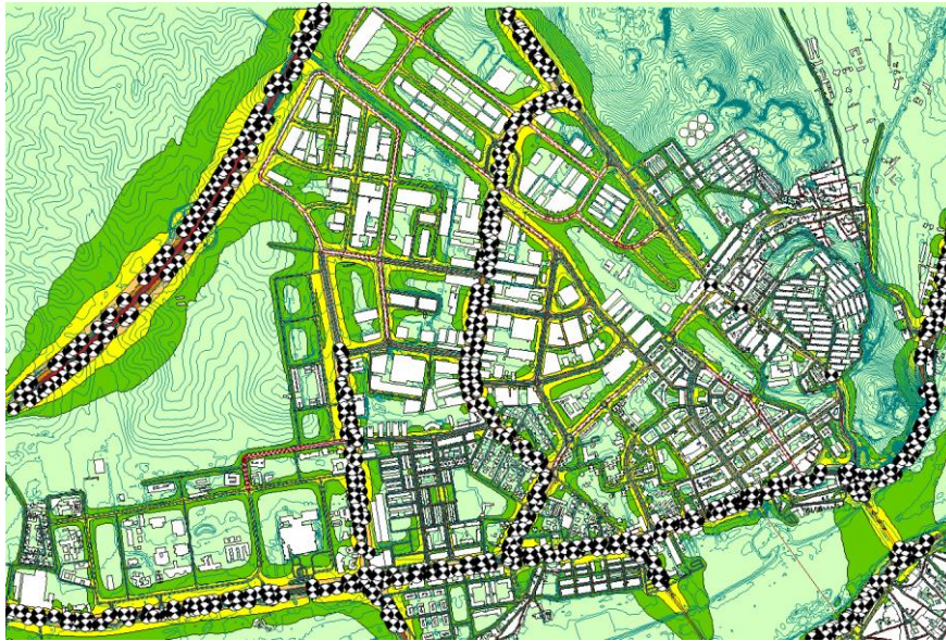
Fig 3 – Set up for the statistical analysis of grid interpolation. Automatic placement of 750 receivers at the 65 dB iso-line
