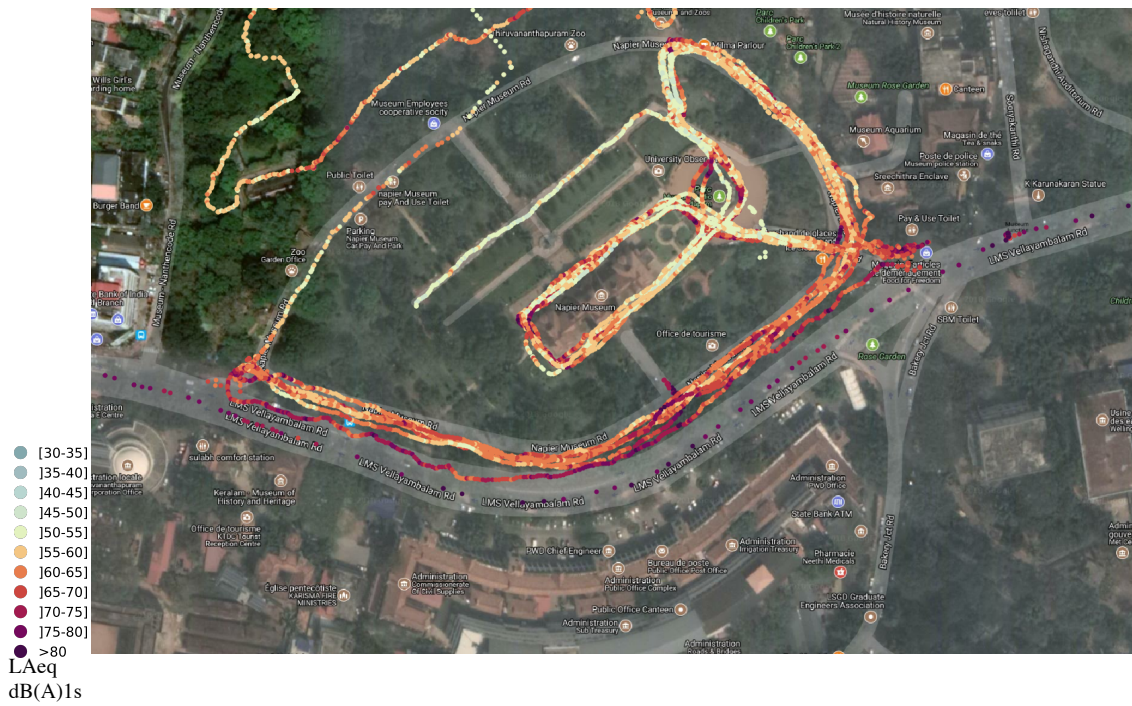
Napier museum Park, Trivandrum (India, 2018). Mobile noise measurements with NoiseCapture. Image: Gwendall Petit (Lab-STICC, noise-planet.org)
