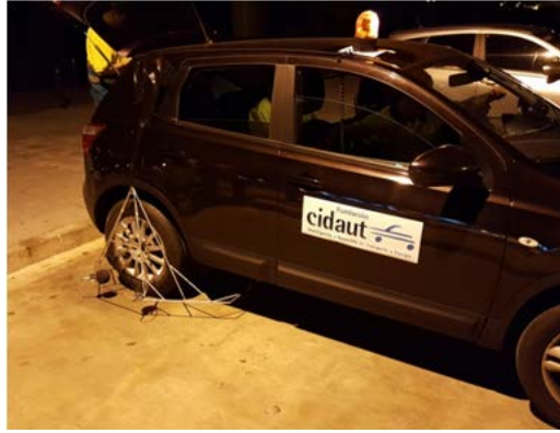
Figure 4.(a) Image of the self-propelled vehicle used for CPX measures
