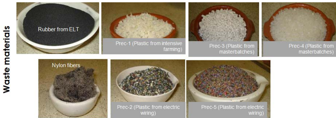
Figure 5. Waste materials used for generating the additives for asphalt mixes.
