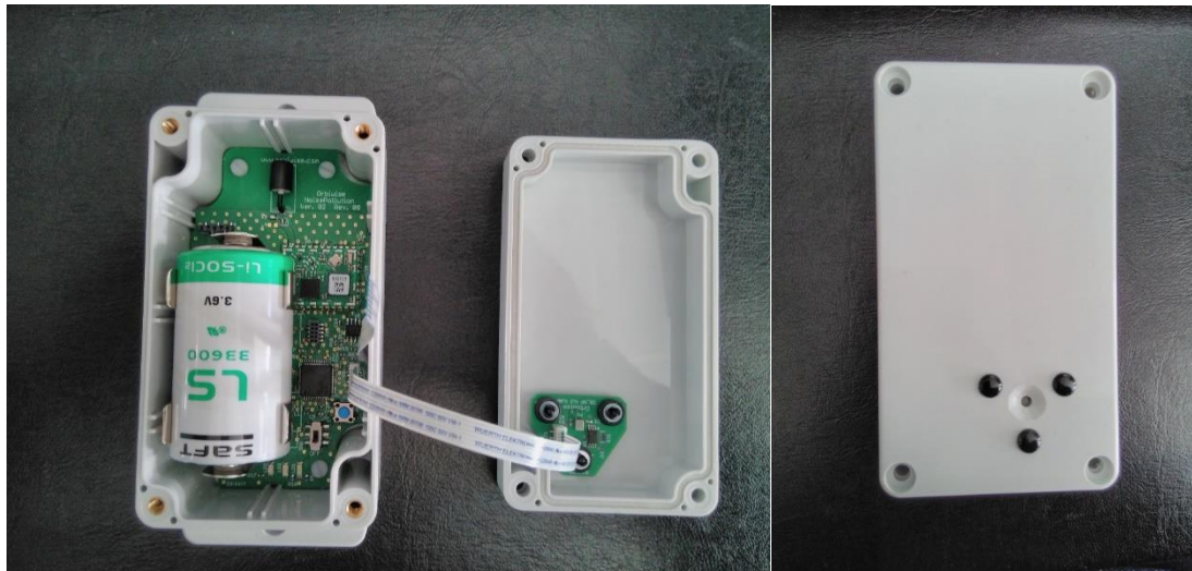
Figure 2: Inner and top view of the autonomous noise sensor
