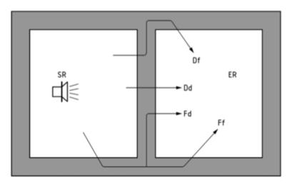
Figure 1: Considered transmission paths in DIN 4109
