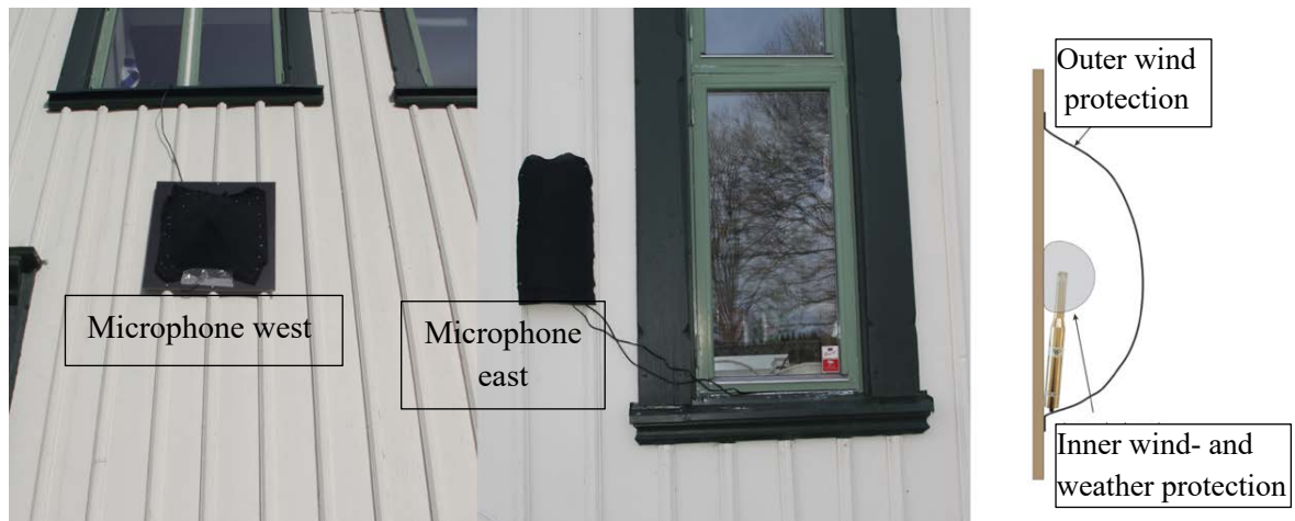
Figure 3. Description of the wind and weather protection used for the measurement series. Calibration of the 6 dB for wall mount and calibration of damping for the wind- and weather protection have been properly handled.
