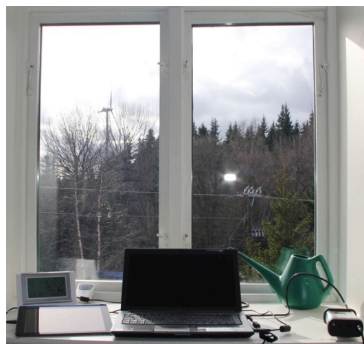
Figure 4. Data collection center placed in the house in the western direction. It is known that the noise impact will be largest in this direction and this room was not occupied.
